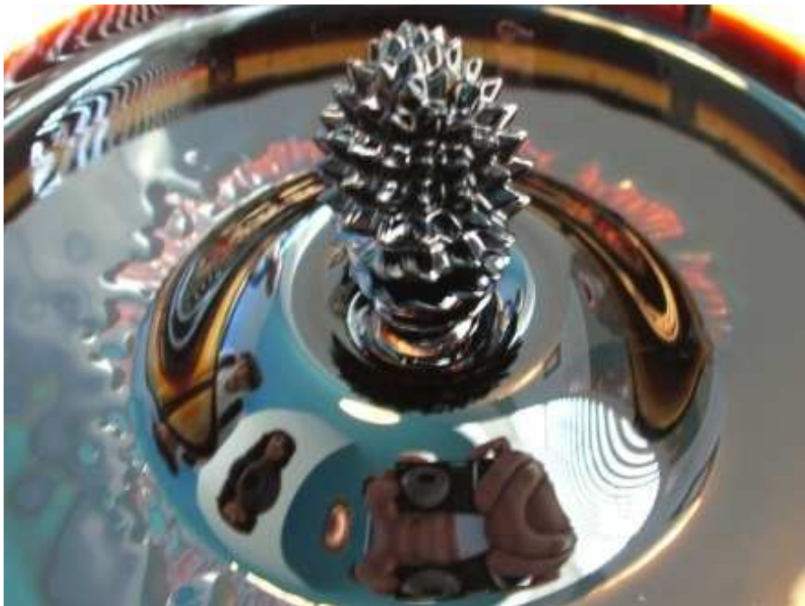
Demonstration of the behaviour of a ferrofluid in a magnetic field
