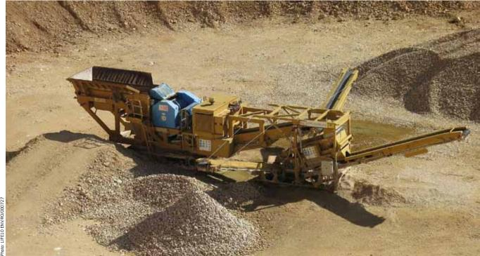
VAL-C&DW developed a mechanical treatment plant that is producing secondary raw materials from construction and demolition waste
