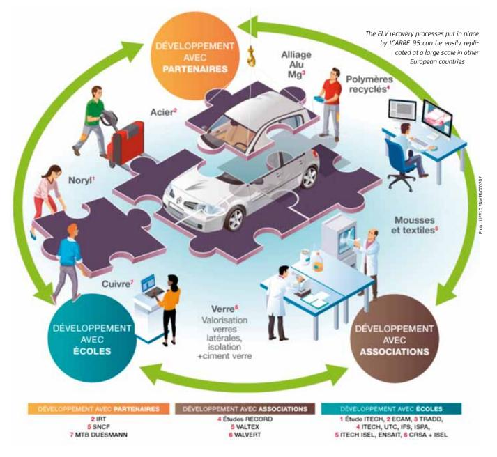
developing innovative techniques to recover and recycle specialised plastic waste from ELVs (see box), for instance, while the projects LIFE CAR-WASTE and PST (see feature article pp 59-61) have demonstrated new post-shredder technology for mechanical sorting, to help bring the overall ELV recycling rate up to 95% by weight.
