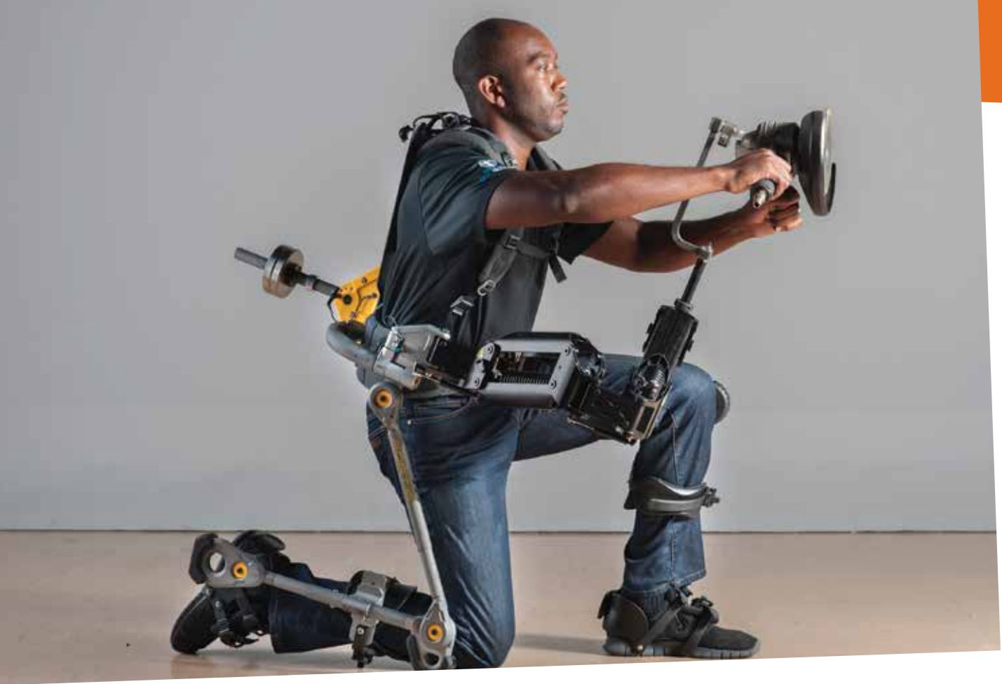
The FORTIS™ exoskeleton allows operators to use heavy tools as if they were weightless. Courtesy of Lockheed Martin. Copyright 2016
