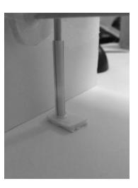
8. Fix the follower with blu-tack or the glue pistol. But be careful! It has to be in touch with the cam in order to transmit the motion.
