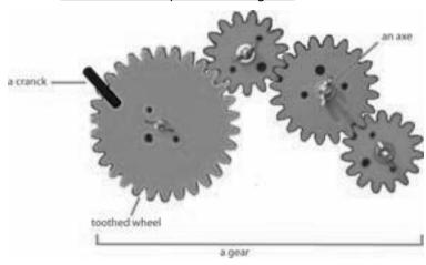
Using these gears, we can accelerate (or decelerate) a motion: it is transmitted but not changed.
